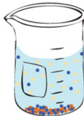
Solid \text{PbSO}_4 and solution with other chemical species (•) and left over \text{SO}_4^{2-} (•)
